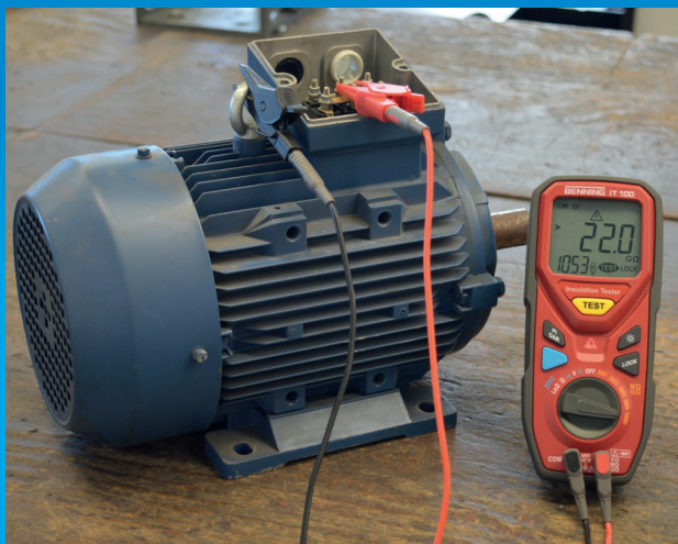
Insulating resistance measurement with 1000 V
