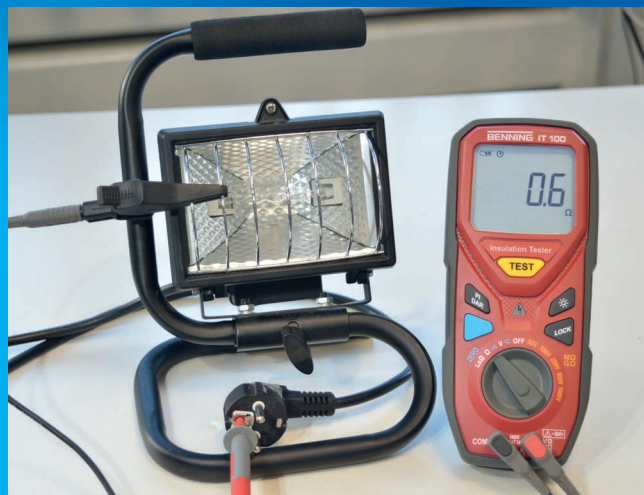
Resistance measurement for testing protective conductor
